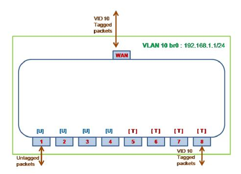
Figure 6.250 Example of LAN Bridge VLAN
